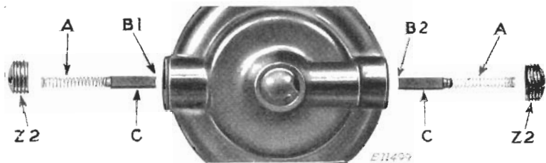
FIG. 25. BRUSHES READY FOR REPLACEMENT (MACHINE 201-3)
