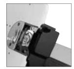
Remaining bobbin thread detector (AE-4)
