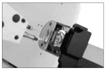
Remaining bobbin thread detector (AE-4)
