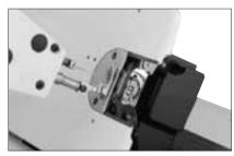
Remaining bobbin thread detector (AE-4)
